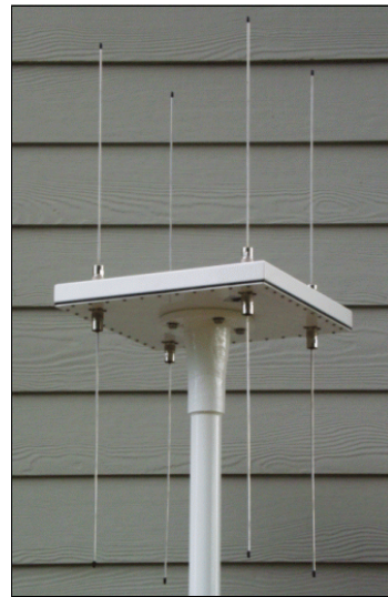
Figure 6 - Mast-Mounted H-Dipole Adcock DF Antenna
