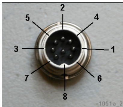
Figure 8 - DF Antenna Chassis Connector Pin Assignments
