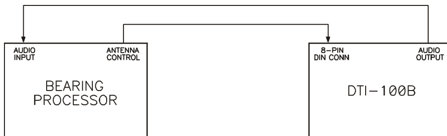
Figure 1 - Test Setup, Bearing Processor Only and DTI-100B
