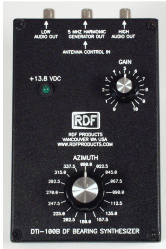
Figure 7 - DTI-100B Control Panel
